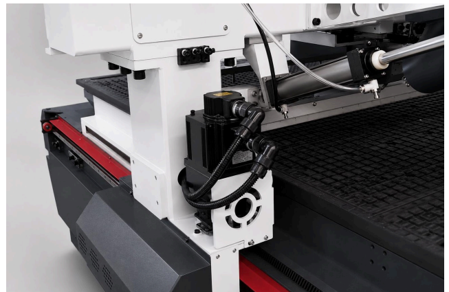
SERVO DRIVE, REDUCER AND HELICAL RACK ON THE X AXIS
