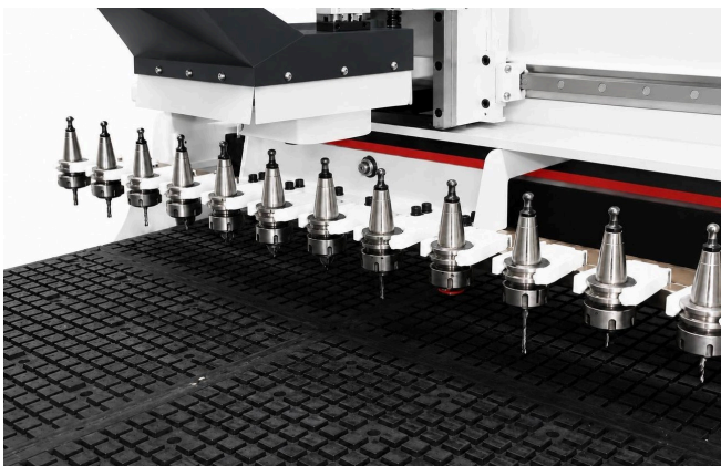
ISO30 TOOL HOLDERS IN THE MAGAZINE, READY FOR AUTOMATIC CHANGE
