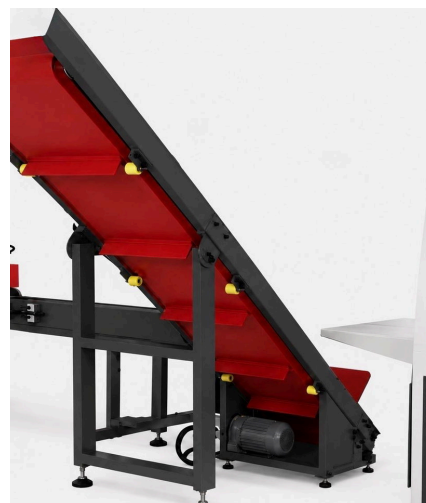
Inclined waste conveyor at the discharge end.
