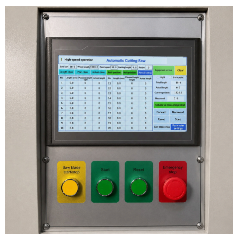
Touch screen with cutting list, planned and actual lengths, position readout and dimensional compensation; 150 lists can be stored and recalled.
