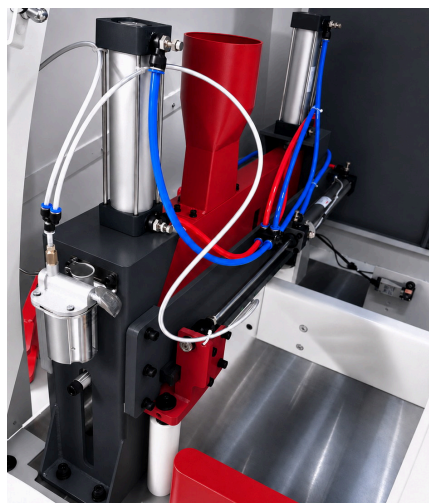
Pneumatic clamping group with upward and side pressure cylinders.
