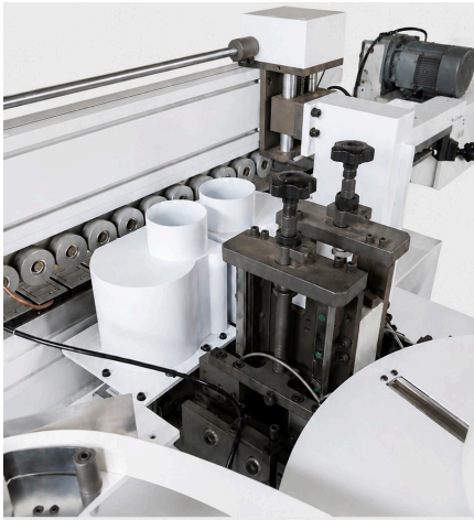
GLUE APPLICATION AND TAPE PRESSING ZONE, WITH THE CHAIN FEED AND PRESSURE WHEELS ABOVE
