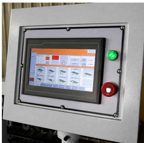
OPERATOR TOUCH SCREEN — STATION SELECTION, TEMPERATURES, FEED SPEED AND PRESSURE BEAM LIFT
