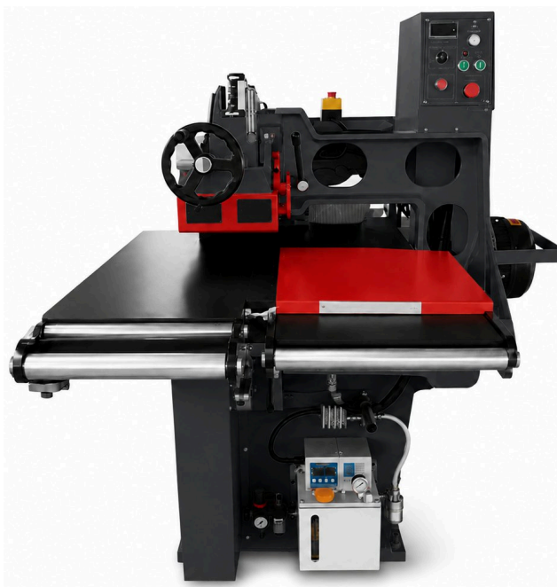
OPERATOR SIDE — INFEED SUPPORT ROLLERS, HANDWHEEL HEIGHT ADJUSTMENT AND CONTROL PANEL
