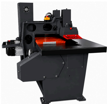
DRIVE SIDE — FEED MOTOR, BELT DRIVE AND PRESSURE BEAM
