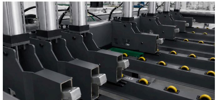
Pusher gripper clamps and transfer castor tracks
