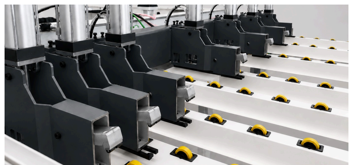
Pneumatic gripper clamps of the pusher beam
