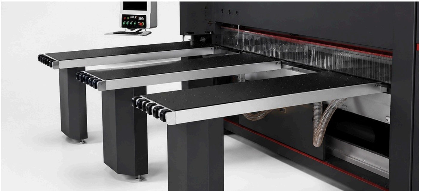
Front view — air-flotation tables, pressure beam and control station
