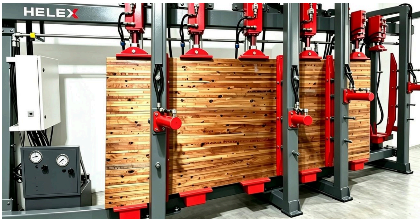
Laminated solid wood packages clamped between the pressing stations.
