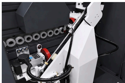
End cutting carriage with tracking guide and tape support
