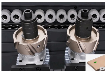
Trimming tooling — carbide cutters for flat and radius profiles
