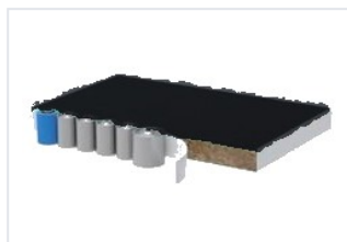
3 Multi-roller pressing Driven + idle rollers
