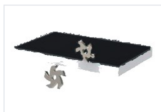
5 Rough trimming Tape surplus removed
