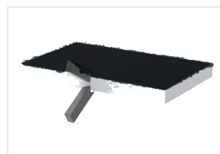
8 Scraping Profile and flat scraper
